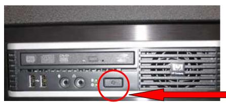
4. If the computer is turned off, it can be turned on using the power button. If machine is locked because someone left themselves logged on, push and hold power button until machine turns off.
